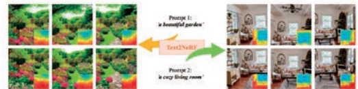
Text2NeRF, a text-driven 3D scene generation framework, combines the neural radiance field (NeRF) and a pre-trained text-to-image diffusion model to generate diverse view-consistent indoor and outdoor 3D scenes from natural language descriptions.
